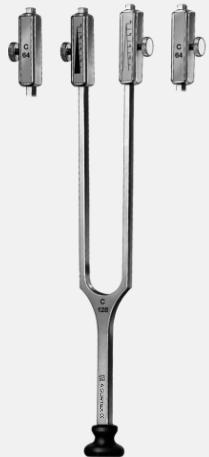
OT-134-00 Rydel-Seiffer Tuning Fork Also For Neurology Frequency With Dampers C 64 Frequency Without Dampers C 128
